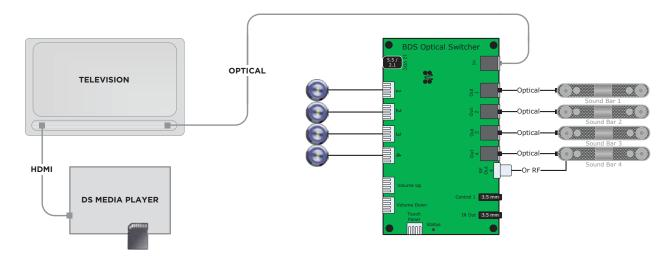
TYPICAL APPLICATIONS DEMONSTRATE 1 TO 4 SOUND BARS BY TURNING THEM ON FOR A PRE-PROGRAMMED TIME. IN SOME CASES THE PRODUCT CAN BE POWERED ON AND THE VOLUME CONTROLLED USING ITS IR REMOTE COMMANDS.
