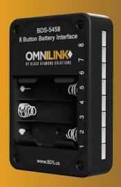
Easily connect 8 buttons wirelessly to a BrightSign Media Player. 3 AA batteries provide a true wireless button with long life. 900MHz wireless frequency (NOT Wi-Fi) is long range and interference free in busy environments.
